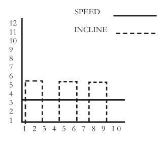
The Rolling Hills Program is designed to vary treadmill elevation while maintaining a constant walking belt speed.
